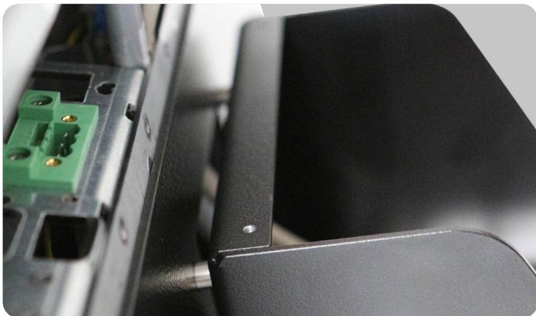
ONCE THE CABLES ARE IN PLACE, ALIGN THE PPC WITH THE MOUNTING SUPPORT AND SECURE IT WITH THE PROVIDED SCREW.
